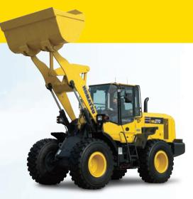
A powerful Komatsu SAA6D107E-2 engine provides a net output of 111 kW 149 HP with up to 10% improved fuel consumption.\* This engine is EPA Tier 4 Interim and EU stage 3B emissions certified.
