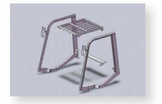
The triplex plate overhead guard is developed using three pieces: left side, right side and top canopy making replacement, when appropriate and authorized, more convenient
