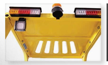
The thin, profiled steel overhead guard helps minimize blind spots, enabling safe and efficient operation.
